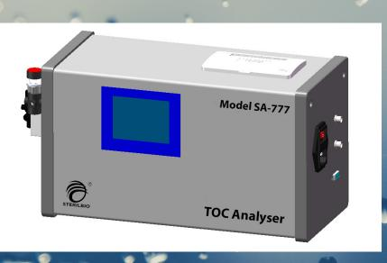
The **STERILBIO Model SA-777 TOC Analyser** is an **on-line and off-line** analyser that uses flow-through UV Oxidation - Conductivity Detection method to determine the TOC levels in Ultrapure water in the Pharmaceutical & Semiconductor Industry. It does not require any reagents or carrier gases for analysis, and hence is very easy to install and use, and maintenance costs are
